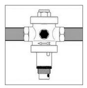
The PRV4PT pressure reducing valve has pressure gauge connections on both sides; both connections are placed on the outlet of the pressure reducing valve.
